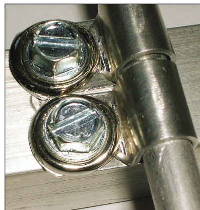
Figure 4 — Detail of a 70 cm director mounted to the boom showing clamps, washers and metal tapping screws.
