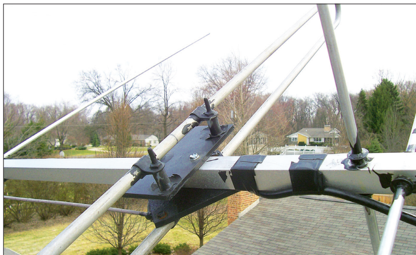
Figure 3 — Elements mounted to boom of 2 meter antenna. The director with Celcon insulator and stud/rod detent washer are clearly visible, as is the driven element feed point with plastic plate.
